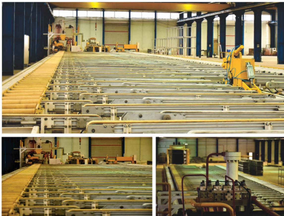
Full automatic conveyor belt table with the smart puller stretch and cutting machine
